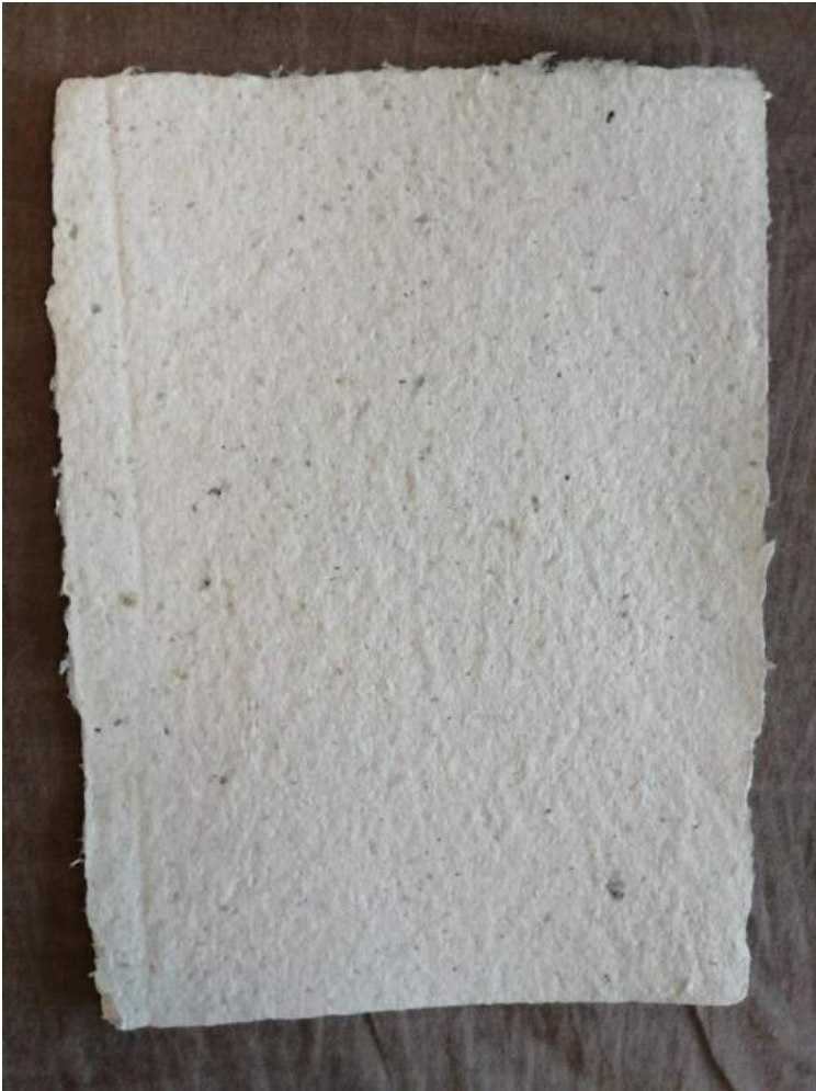
Sample 5. Paper made out of old magazines, using blender and the sponge method for paper-forming
