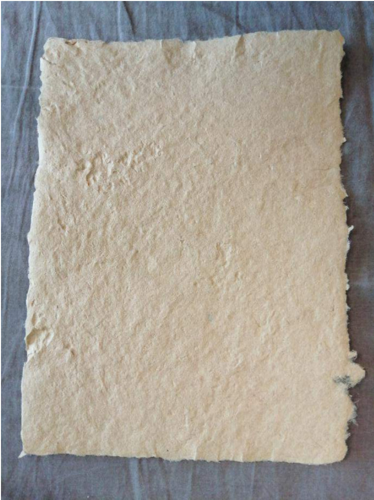
Sample 7. Paper made out of old paper bags, using blender and a new sponge method
